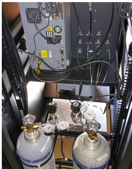
Earth Networks, an AEM brand, and Scripps Institution developed a system for calibrating gas analyzers and function monitoring. The system includes a calibration box and two air tanks.
