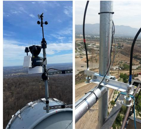
AEM GHG Observation Network installation including a Vantage Pro2 weather station and two air sampling lines.
