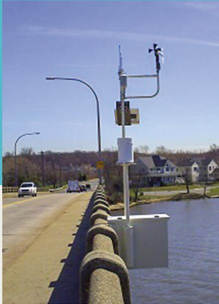
Mounting options include, pole, telemetry cabinet, and mounting plate.
